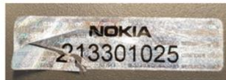
Figure 13: Tamper-evident label: broken (close-up view)
