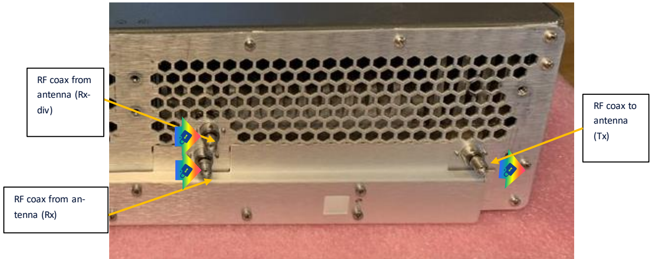
Figure 7: MPT-HLC ports and interfaces on Backplane
