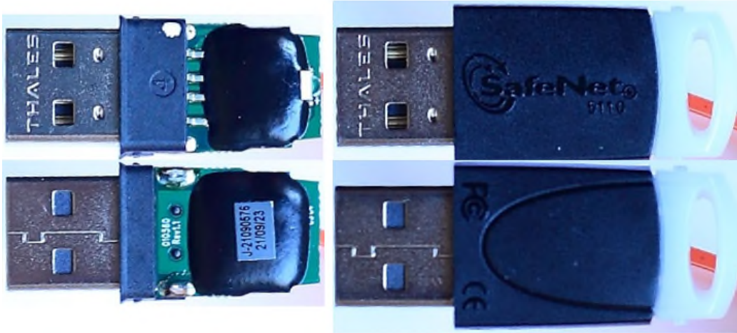
Figure 1 – 'eToken 5110+ FIPS' Crypto Boundary
