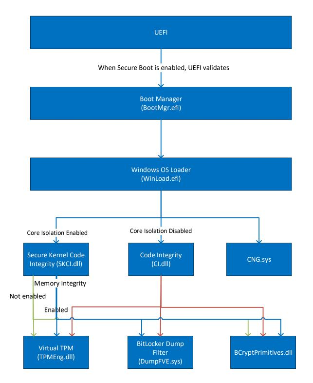
The integrity of Boot Manager is verified by UEFI when Secure Boot is enabled and by the Boot Manager itself.
