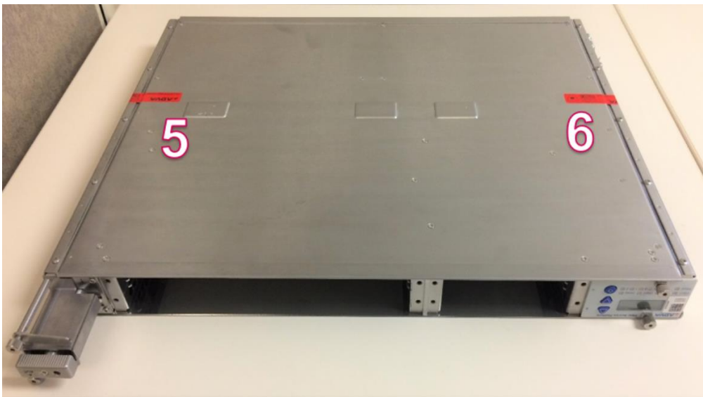
Figure 23: Placement of seals SH1HU-R/PF front-bottom
