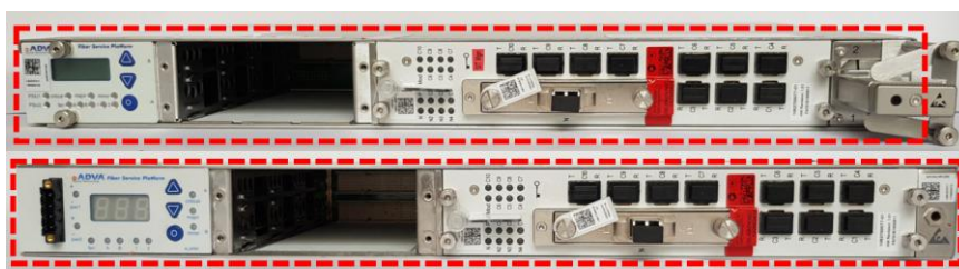
Figure 6: 10TCE mounted in shelf SH1HU (red dotted line indicating Cryptographic Boundary)
