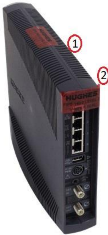
Figure 2 – Back View of the HT2300
