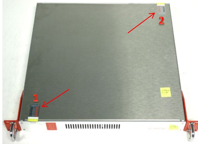
Figure 5: E Variant Tamper-Evident Seal Locations (Top, Back) (Red Arrows)
