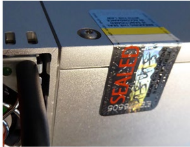
Figure 9: Tamper-Evident Seal X-Module Back
