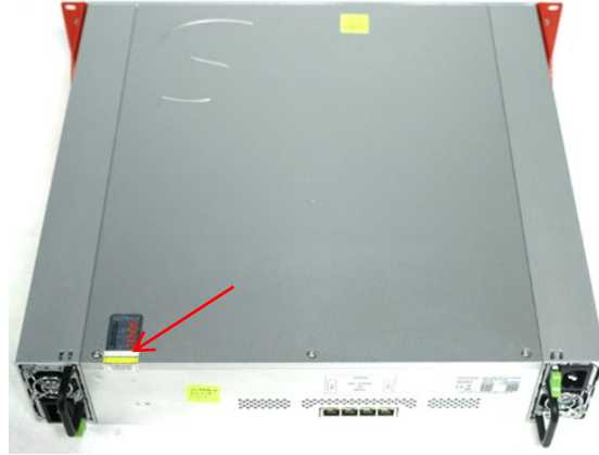
Figure 8: X Variant Tamper-Evident Seal Location (Top, Back) (Red Arrow)
