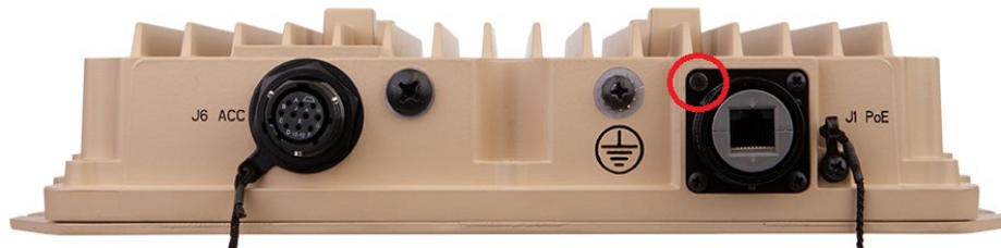
Figure 12 – Tamper-Evident Pin Location for RF-7800W-OUxx1 (12069-3035-02)
