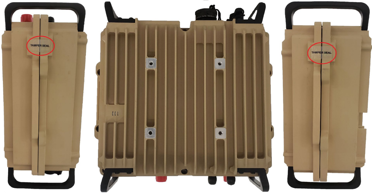
Figure 9 – Tamper-Evident Seal Locations for RF-7800W-RPxx1 (12069-5010-02)
