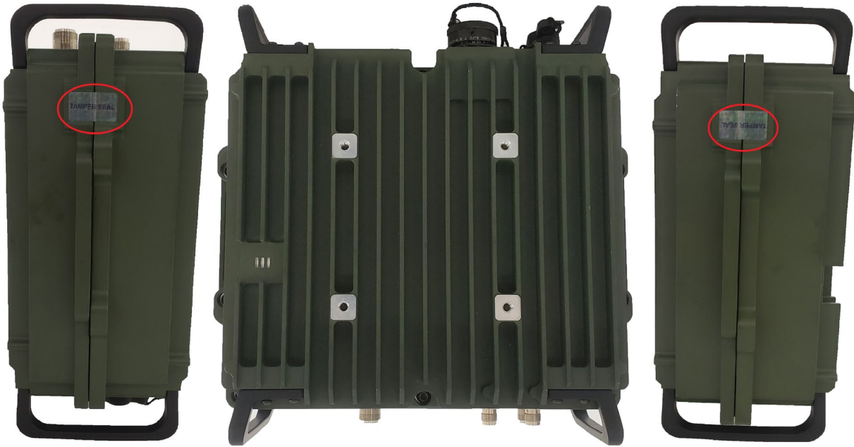
Figure 8 – Tamper-Evident Seal Locations for RF-7800W-RPxx0 (12069-5010-01)
