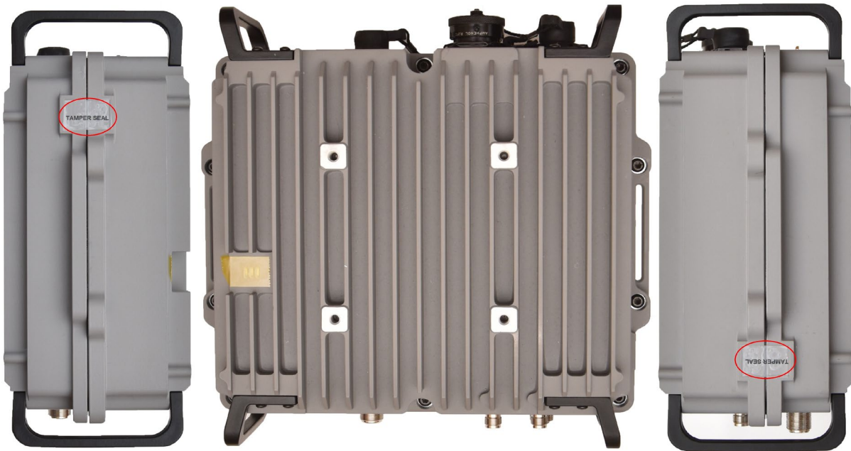
Figure 10 – Tamper-Evident Seal Locations for RF-7800W-RPxx3 (12069-5010-04)
