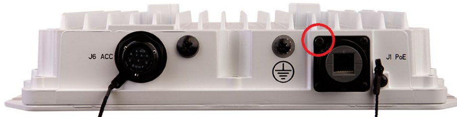
Figure 13 – Tamper-Evident Pin Location for RF-7800W-OUxx2 (12069-3035-03)
