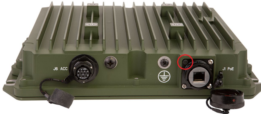
Figure 11 – Tamper-Evident Pin Location for RF-7800W-OUxx0 (12069-3035-01)
