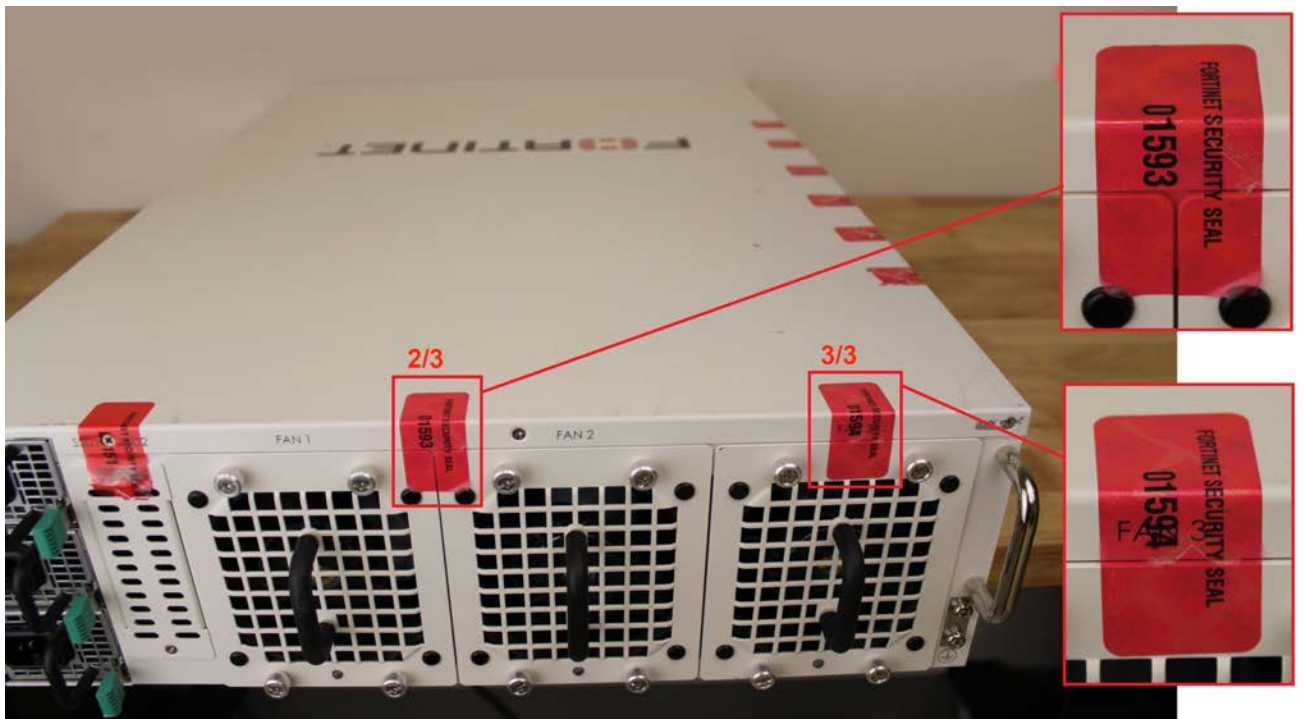
Figure 3 - FortiGate-6300F/6301F/6500F/6501F external enclosure seal 2 and 3, top, rear
