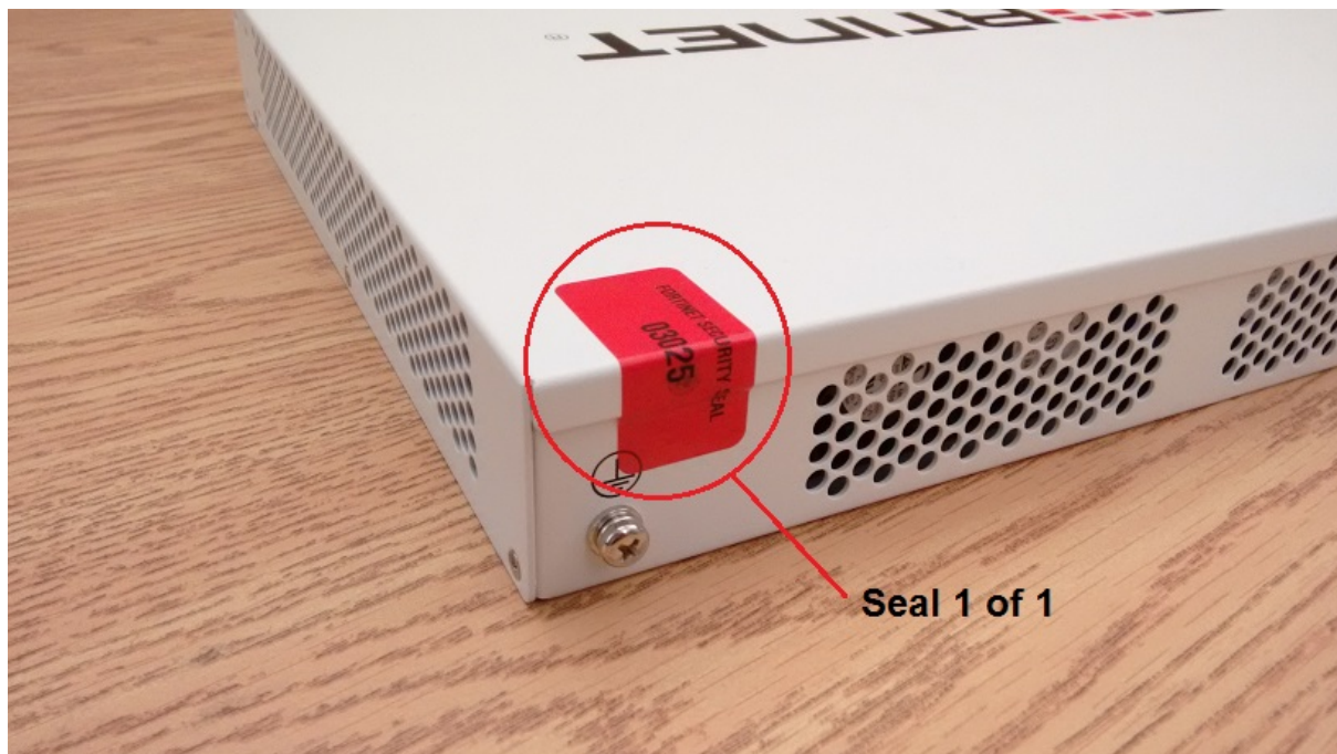
Figure 4 - FortiGate-201E external enclosure seal, top, rear
