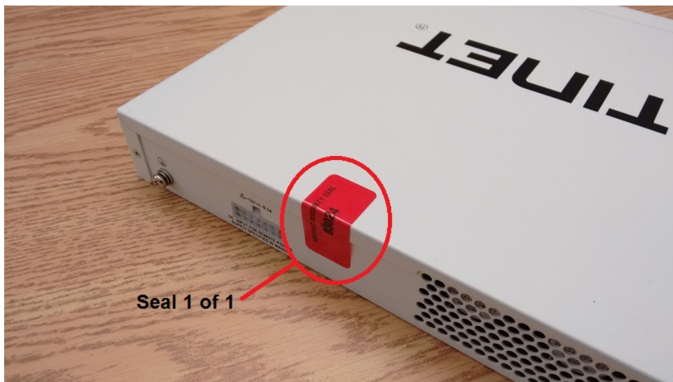
Figure 10 - FortiGate-101E external enclosure seal, top, rear
