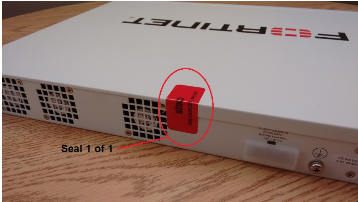
Figure 15 - FortiGate-600D external enclosure seal, top, rear
