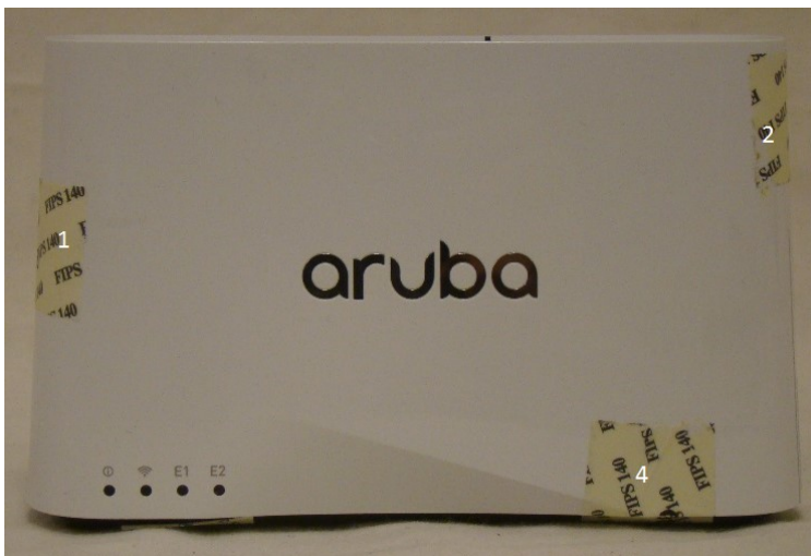
Figure 13 – Front View of AP-203RP with TELs
