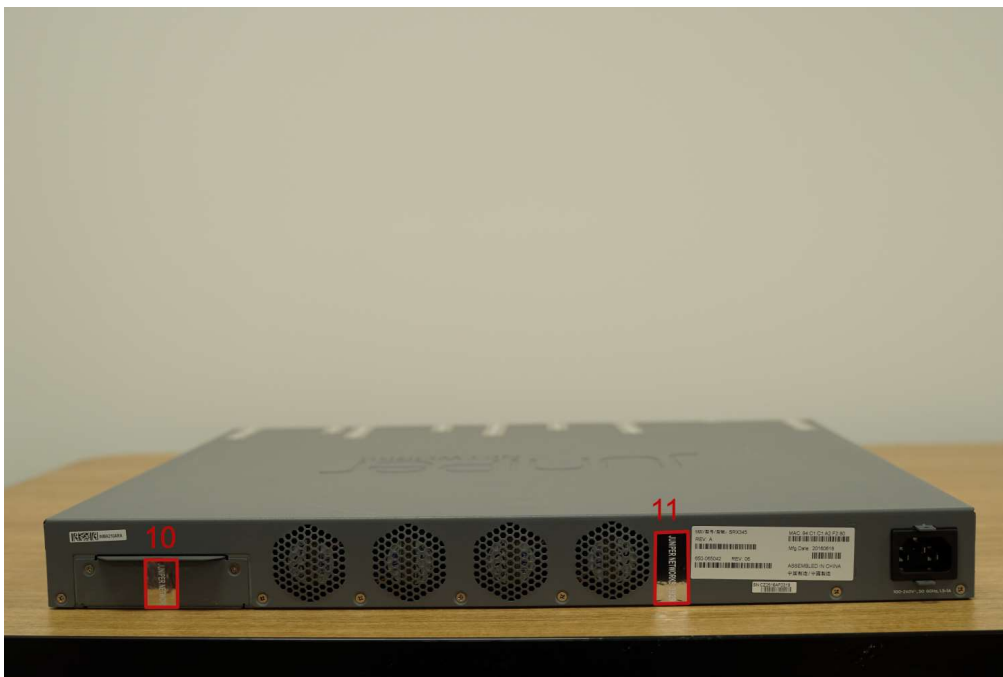
Figure 13 – SRX 345 Tamper-Evident seal placement (LHS)
