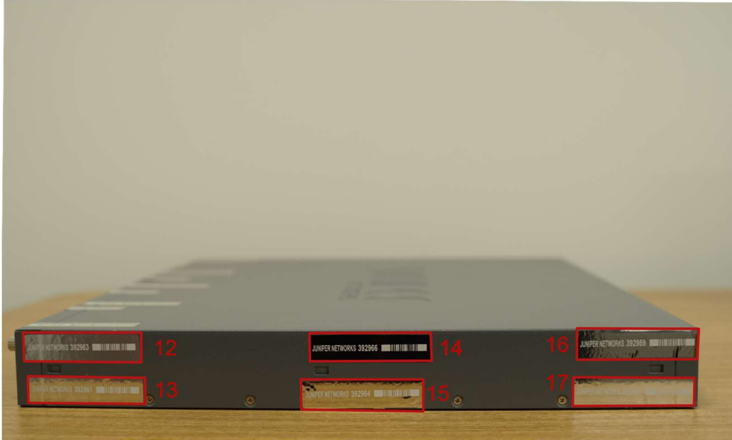
Figure 19 - SRX345 Dual-AC Tamper-Evident seal placement (RHS)
