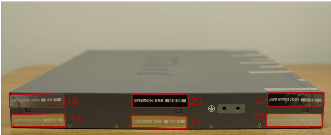
Figure 19 - SRX345 Dual-AC Tamper-Evident seal placement (RHS)
