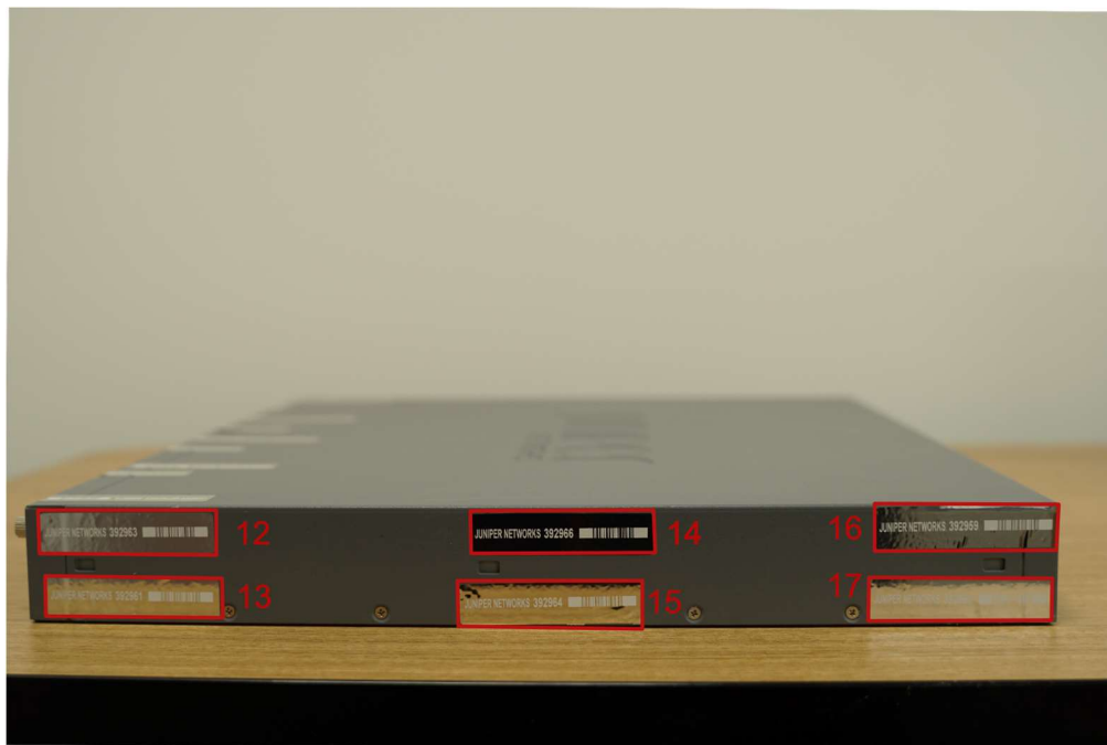
Figure 13 – SRX 345 Tamper-Evident seal placement (LHS)
