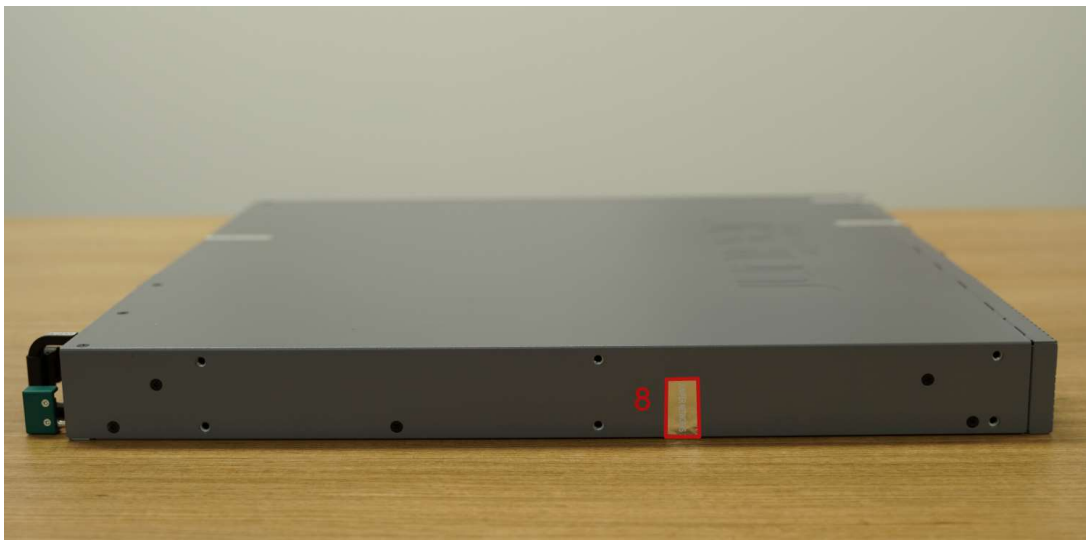
Figure 23 – SRX1500 Tamper-Evident seal placement (RHS)
