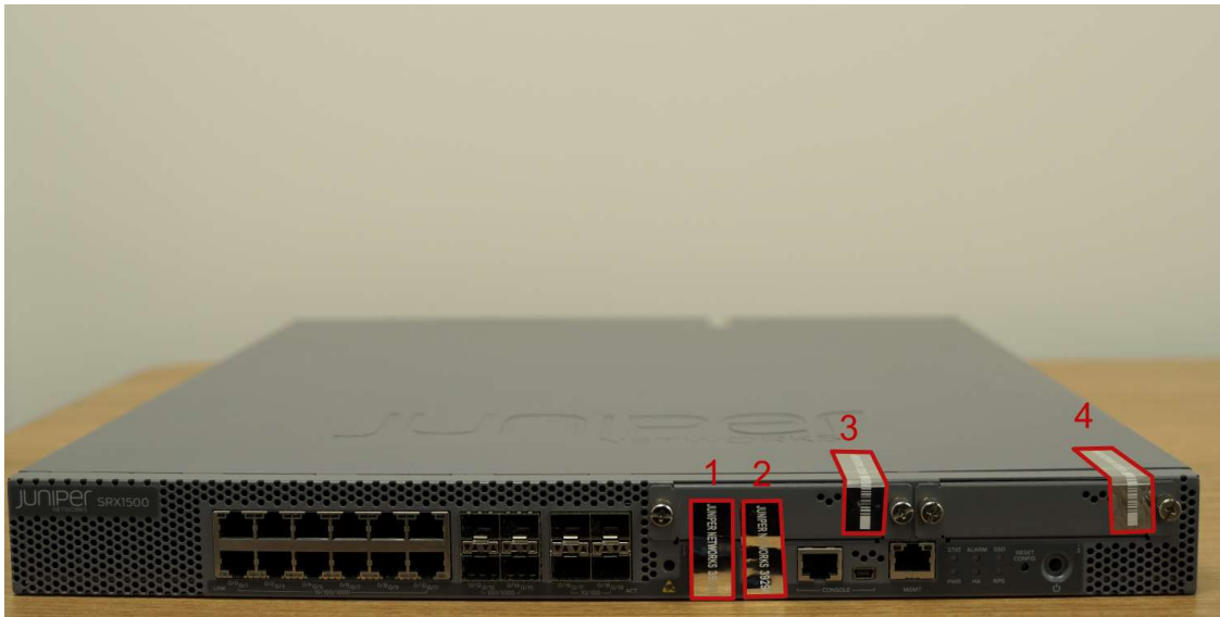
Figure 21 – SRX1500 Tamper-Evident seal placement (Rear)
