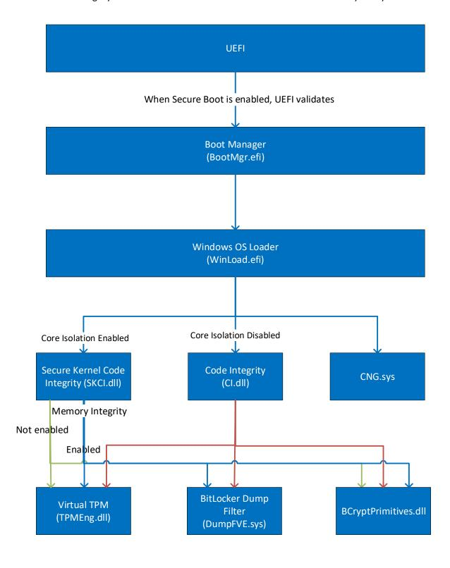
The integrity of the Secure Kernel Code Integrity module is checked by the Windows OS Loader. If VSM is enabled, then the Secure Kernel Code Integrity module is then invoked by the Code Integrity module to check the integrity of user mode binaries (including BCRYPTPRIMITIVES.DLL) as they are loaded. If HVCI
