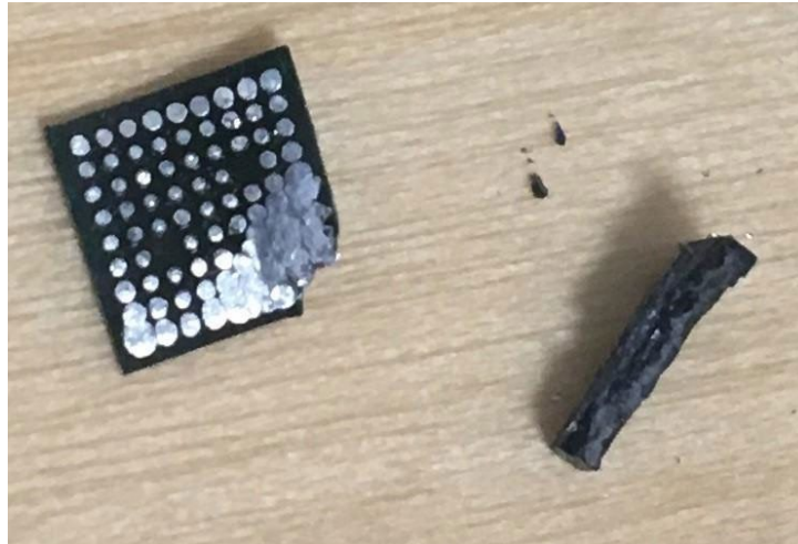
Figure 4- Tamper Evidence and damage to the module
