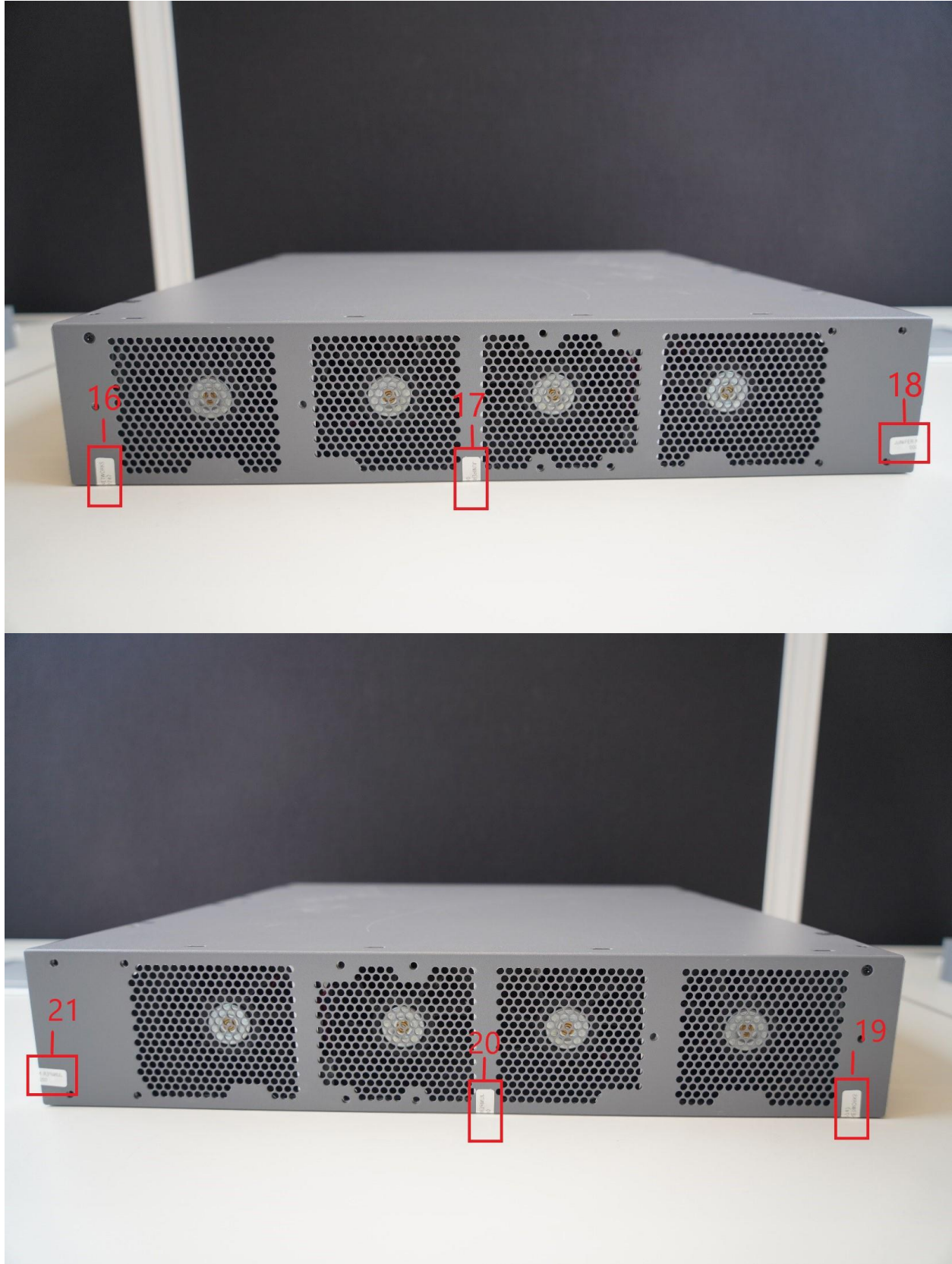
Figure 27 – SRX550M Tamper-Evident Seal Placement (Side, Three a side (6) Seals: TEL 16-21)
