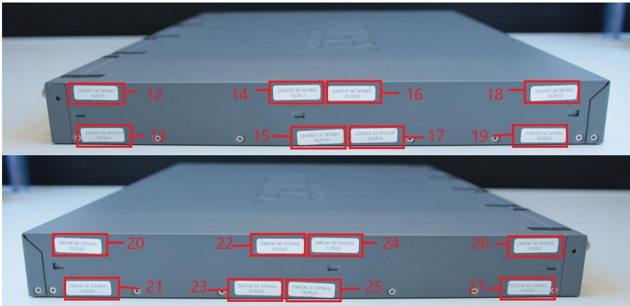
Figure 24 - SRX340/SRX345 Tamper-Evident Seal Placement (Right Side Panels, Eight on each side – Sixteen (16) Seals: TEL 12-27)
