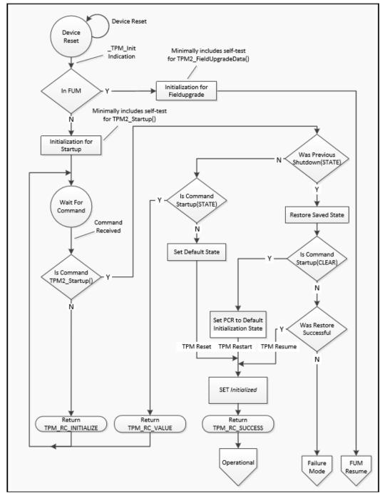
For self-testing, if a command is received that requires return of a value that depends on untested functions, the TPM shall test the required functions before completing the command. The Virtual TPM executes all of the self-tests directly from its "DIIMain" function, which occurs prior to "\_TPM\_Init" in the diagram. Furthermore, the "Device Reset" section of the diagram refers to when the Virtual TPM library is reloaded.
