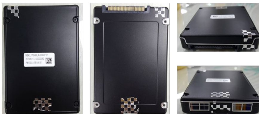
Figure 4. Example of Signs of Tamper
