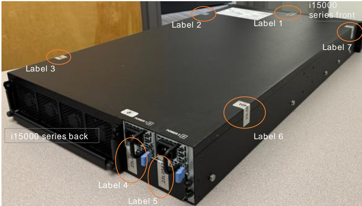
Figure 13 - Tamper labels on BIG-IP i15600, BIG-IP i15800, and BIG-IP i15820-DF. 1 label on the front, 4 labels on the sides, 2 tamper labels shown circled in orange to mark with evidence the unauthorized removal of the fan tray and PSUs (replaceable items) that give access to replaceable storage drives.
