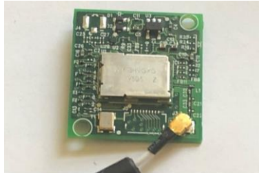
Figure 1 - Module's Hardware Component (Zebra WLAN Core)
