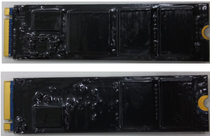
Exhibit 4 - Specification of the PS5012-E12 M.2 2280 NVMe NAND FLASH SSD Series Cryptographic Boundary (From top to bottom: top side, bottom side).
