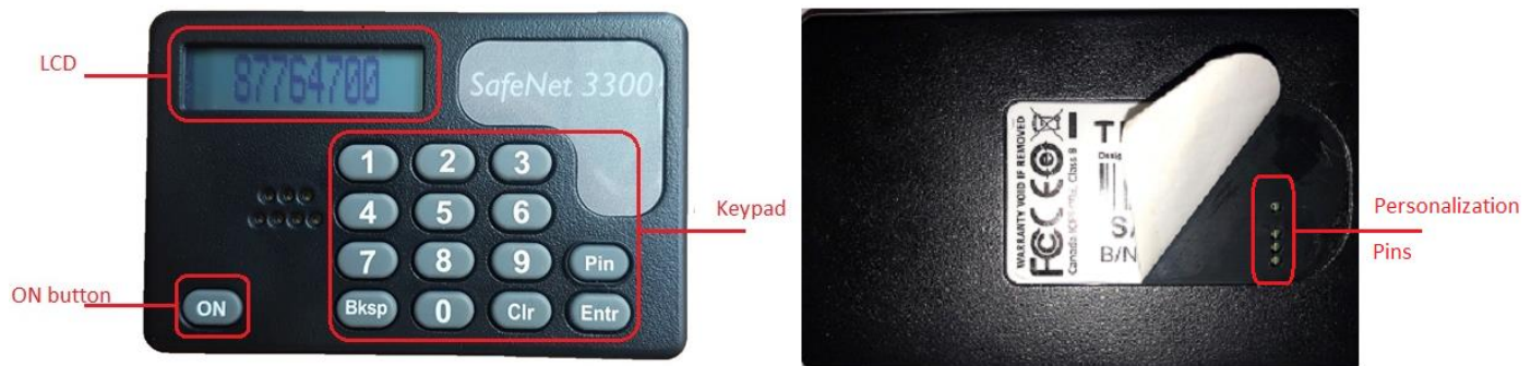
Figure 3-1: Safeword3300 Platinum V2F Cryptographic Module physical interfaces
