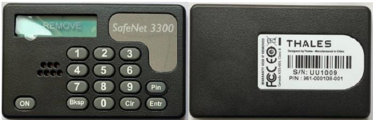
Figure 2-3: Safeword3300 Platinum V2F HW 1.0 with standard markings
