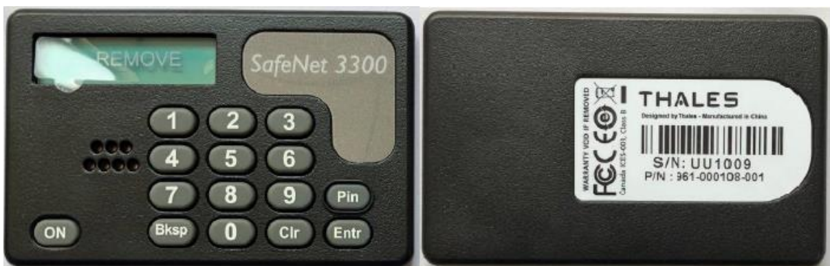
Figure 2-1: Safeword3300 Platinum V2F Cryptographic Module cryptographic boundary
