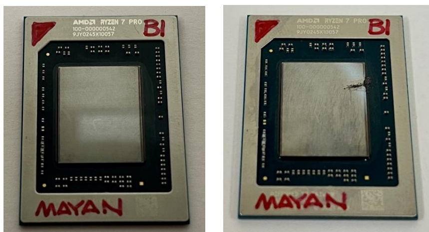
Figure 4: Module before Tampering (Left) and after Tampering (Right)
