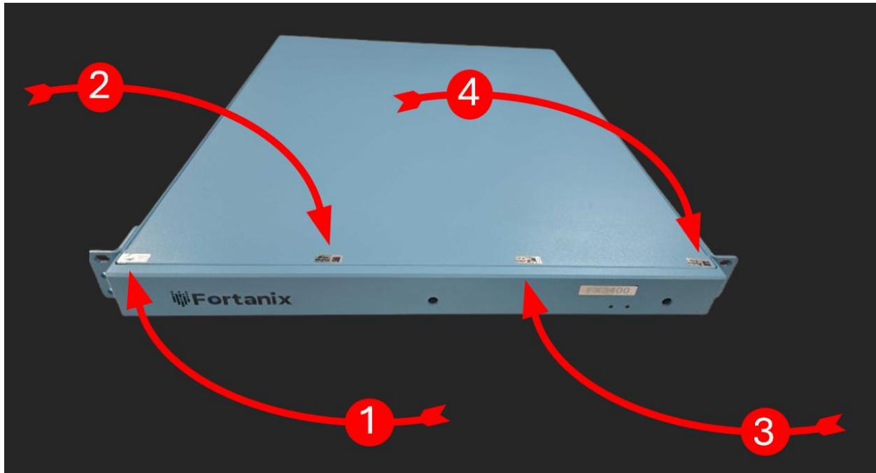
Figure 13: Tamper Evident Label Positions on FX3400-T, FX3400-F, FX3500-T and FX3500-F
