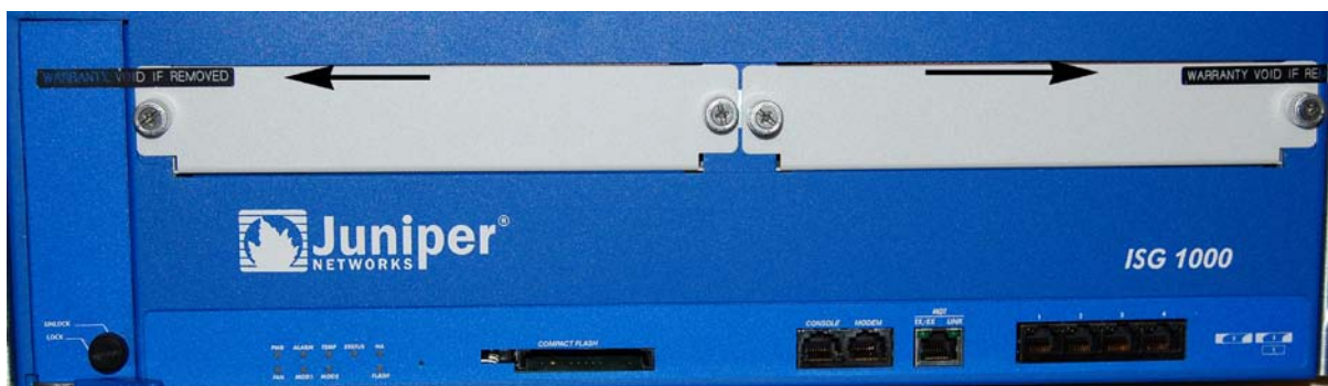
Fig. 1: Front of the ISG 1000, with location of tamper evident seals
