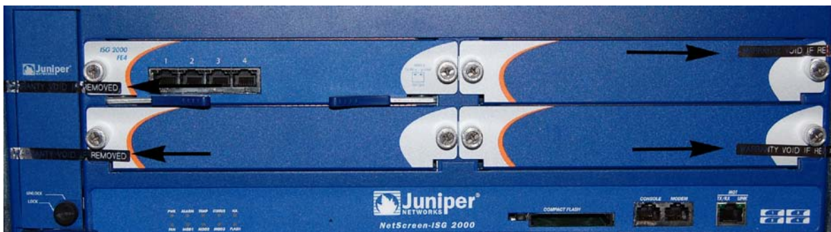
Fig. 3: Front of the ISG 2000, with location of tamper evident seals
