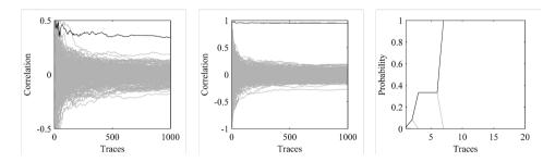
Super simple example already given in the DPA book. (Left: single bit attack, ca. 160 traces; Middle: HW based differential attack, ca. 20 traces; Right: template based differential attack, ca 6 traces)
