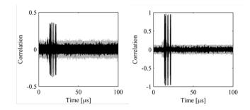
(Left: very simplistic single-bit leakage model, Right: device appropriate leakage model).
