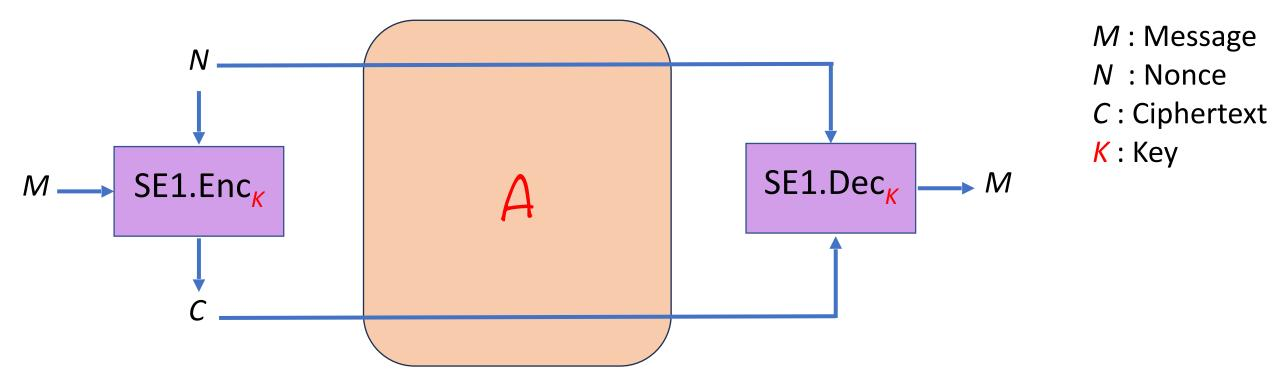
Scheme SE1 specifies encryption algorithm SE1.Enc and decryption algorithm SE1.Dec. Note that the decryption algorithm needs and gets the nonce *N* as input as per the AE1 syntax.
