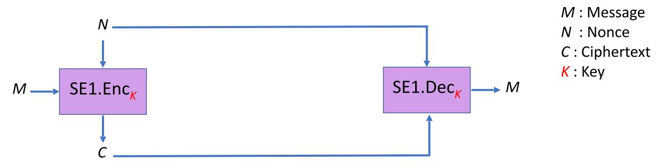
Scheme SE1 specifies encryption algorithm SE1.Enc and decryption algorithm SE1.Dec. Note that the decryption algorithm needs and gets the nonce *N* as input as per the AE1 syntax.
