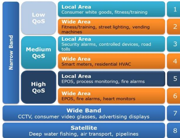
Figure 3: Application categories, based on range, bandwidth and QoS.
