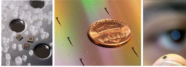
**Figure 1.** Previous generations of passive UHF RFID chips on a salt cellar, a silicon wafer, and a finger-tip.
