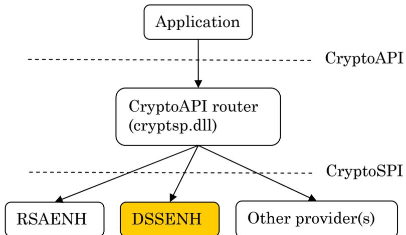
Figure 2 Relationship to other components in Windows CryptoAPI system – cryptographic module shown in gold
