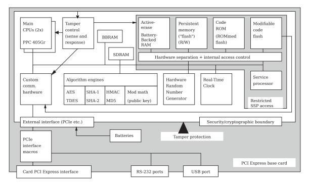
Figure 3: Module hardware architecture, with directly connected components on the hosting PCIe board
