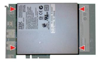
Figure 4: The module as mounted on its PCIe board
