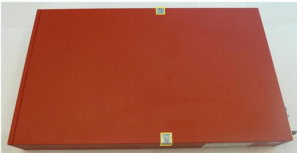
Figure 4 - Tamper Evident Labels On Chassis (outlined in yellow for emphasis)
