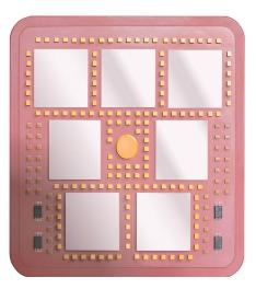
Figure 2: z10 EC Processor Unit MCM with CPACF COP chips
