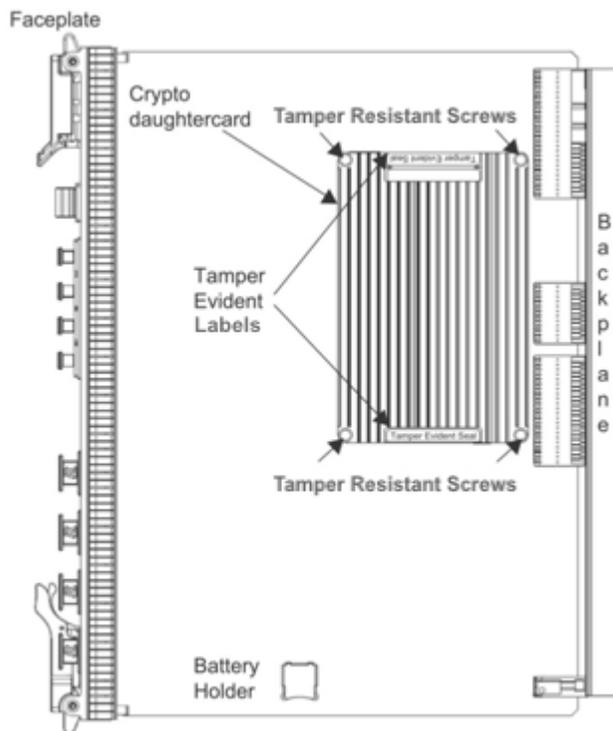
**Figure 4 – Circuit Pack with Module Installed (Tamper-Evident Screws and Labels Shown)**
