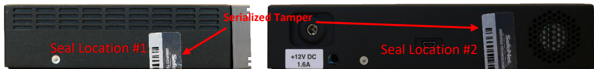
Figure 3-1. Tamper Evident Label Locations
