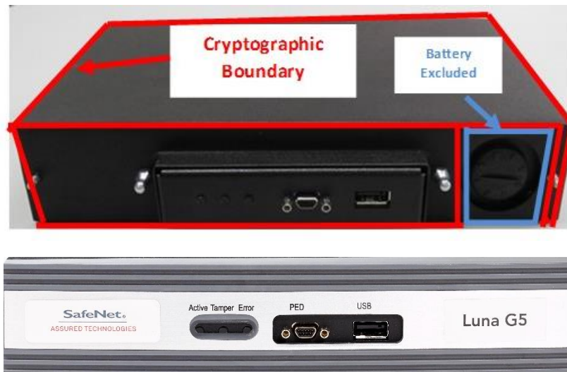
Figure 2-2. Luna G5 Cryptographic Boundary (with front bezel removed)
