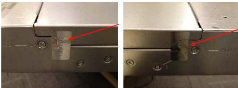
Figure 10 – Tamper-Evidence Labels on Side of ESKM
