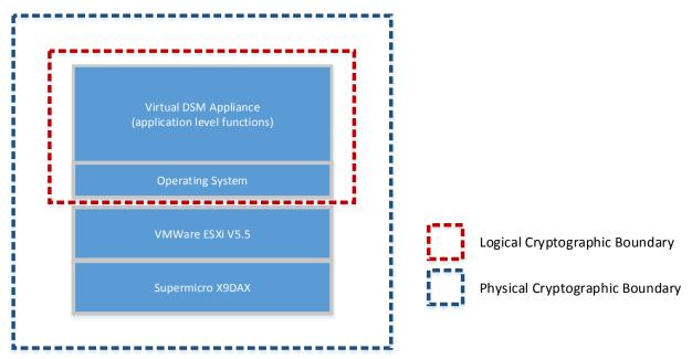
Figure 2. Logical Cryptographic Boundary
