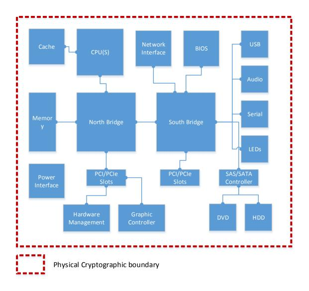
Figure 1 - Physical Module Cryptographic Boundary
