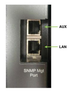
Figure 11 – RJ45 Ethernet close-up
