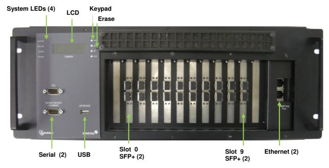
Figure 8 - Front View of the CN8000 Encryptor
