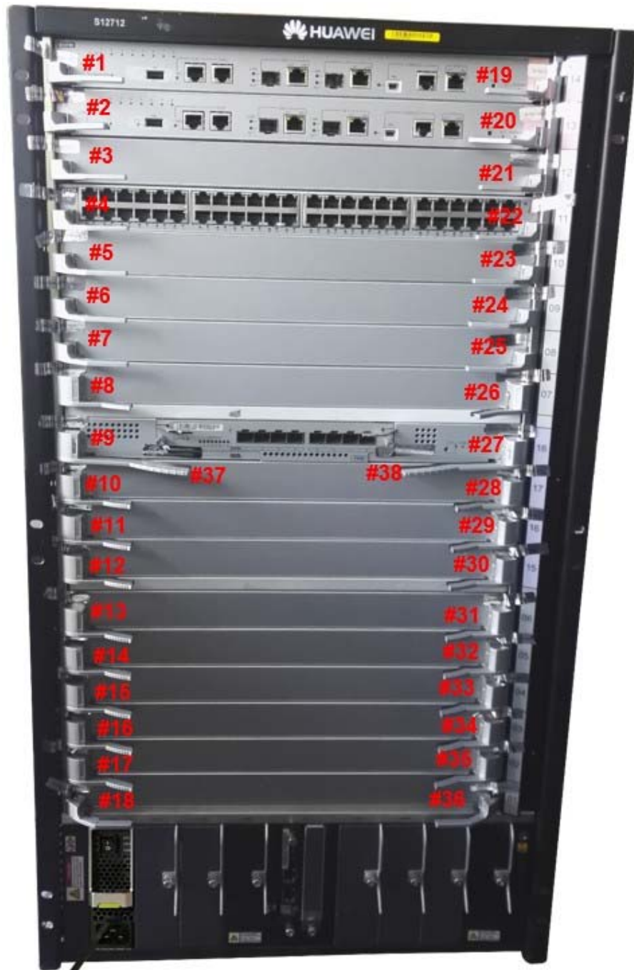
Figure 7-5: Tamper Seal Locations - Front
