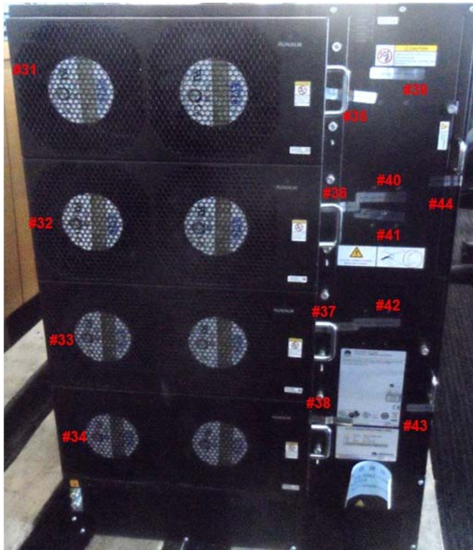
Figure 7-4: Tamper Seal Locations - Back
