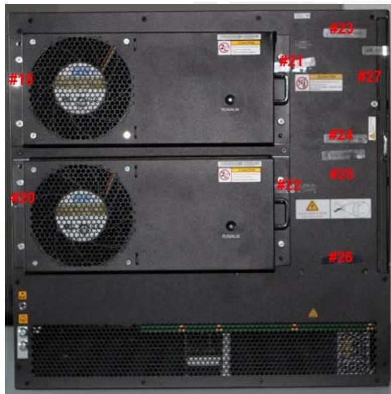
Figure 7-2: Tamper Seal Locations - Back
