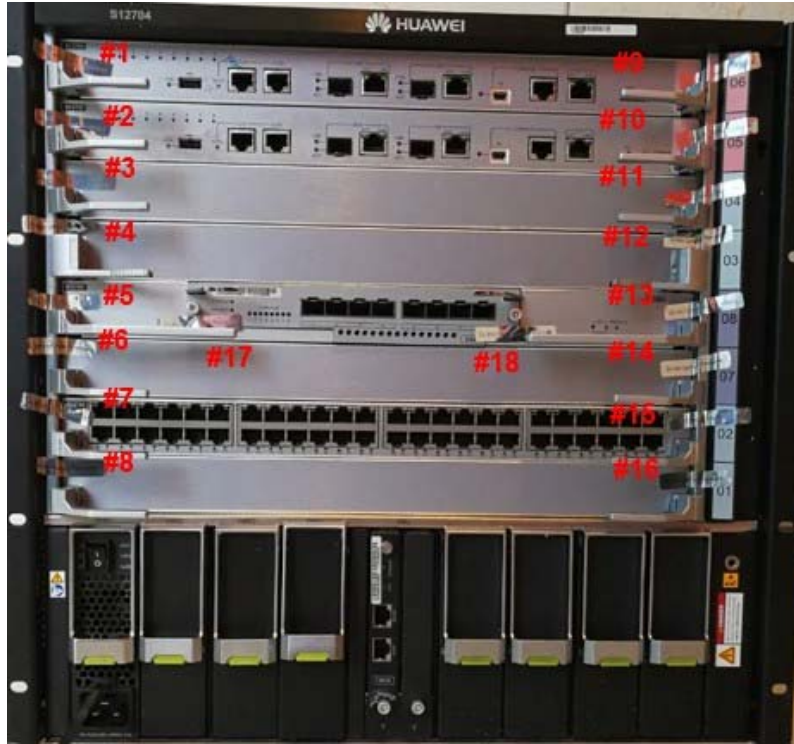
Figure 7-1: Tamper Seal Locations - Front
