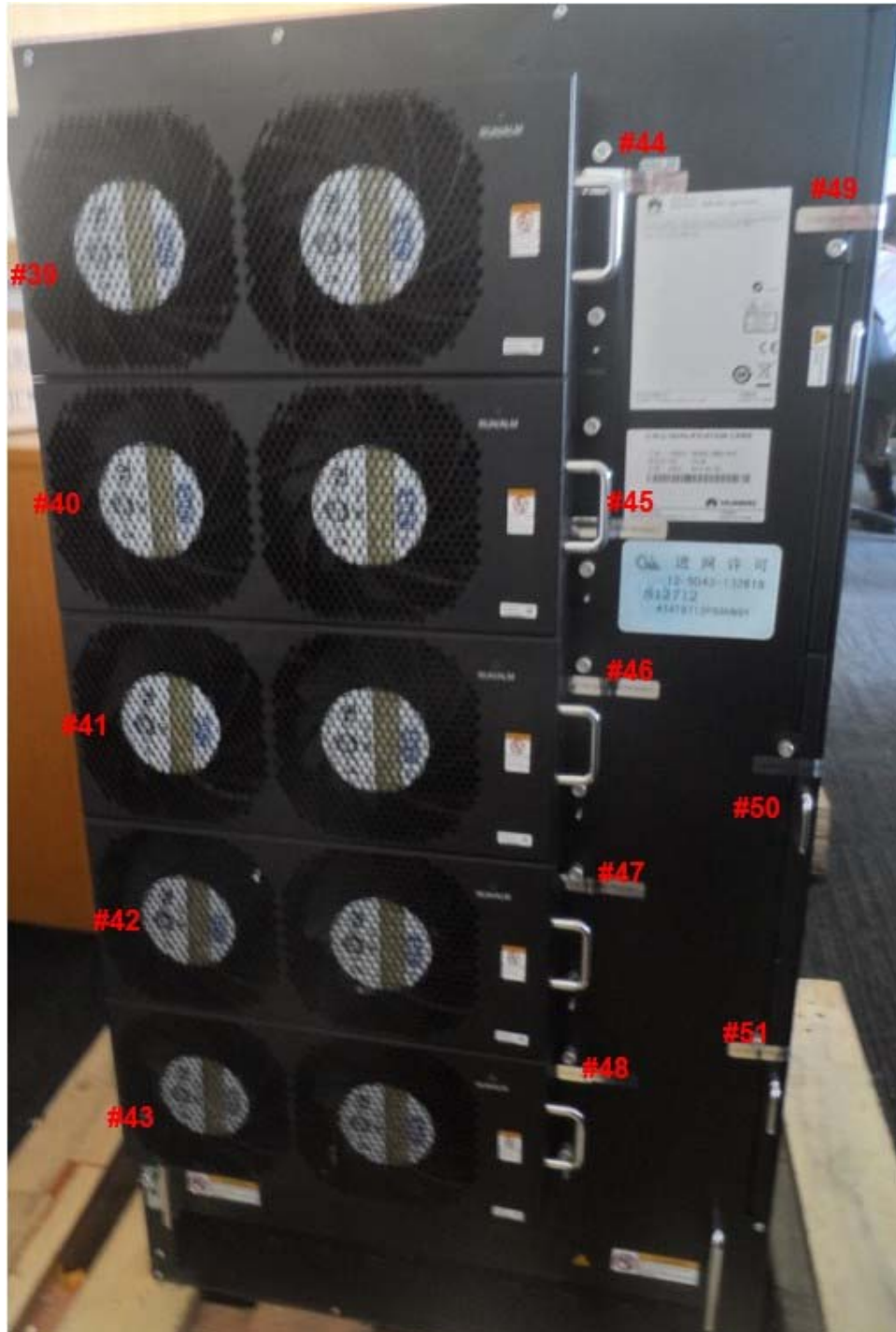
Figure 7-6: Tamper Seal Locations - Back
