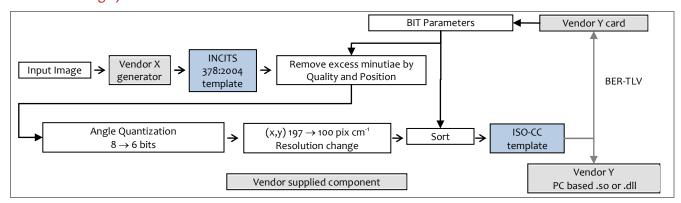
Figure 3 – Conversion of INCITS 378 to ISO/IEC 19794-2 card data
